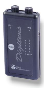
DIGITENS is an advanced hand held dual Channel Pocket model TENS in the field of Electrotherapy. The microcontroller based circuitry has six preprogrammed output modes that can be selectable by a soft touch key. It has 15 mins built in timer and it will be operated by battery/mains.
